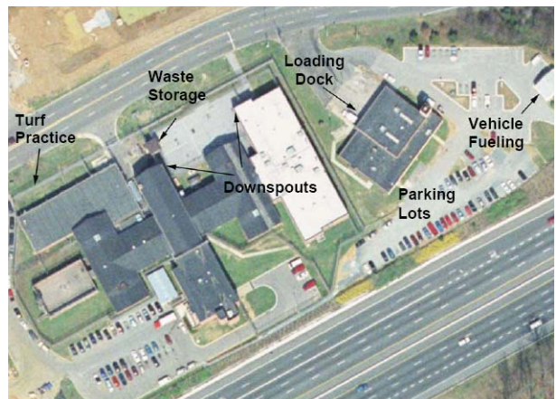
Impervious surfaces contribute pollutants to rain water runoff.
