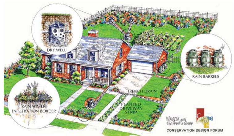
Best Management Practices on residential lots may include rain barrels, rain gardens, and native landscape systems.
