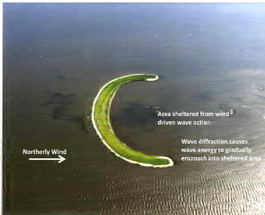
Photograph 9-3. Example of Reduced Wave Action and Sediment Resuspension
