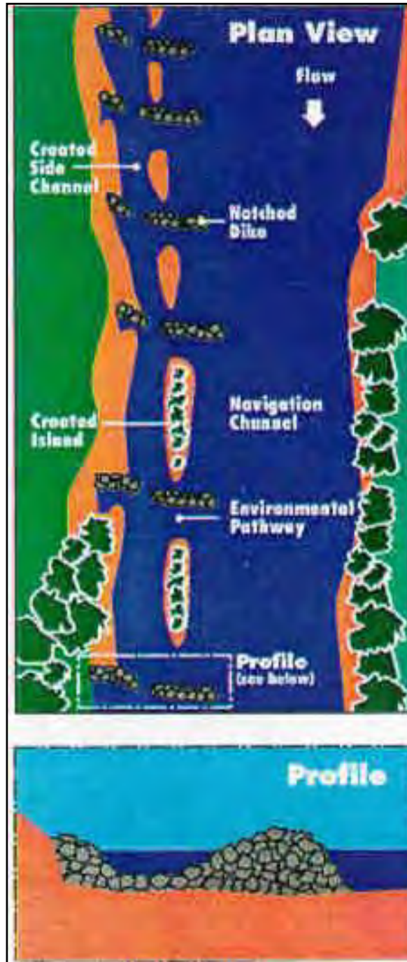
Figure 7-1. Wing Dam Notching
