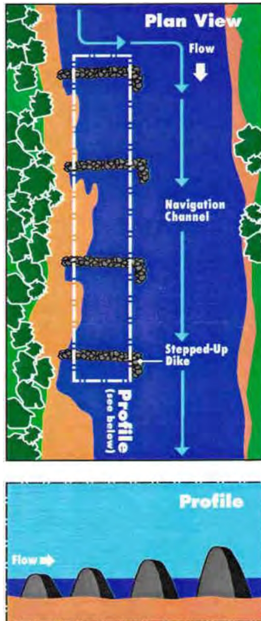
Figure 7-7. Stepped Up Dikes
