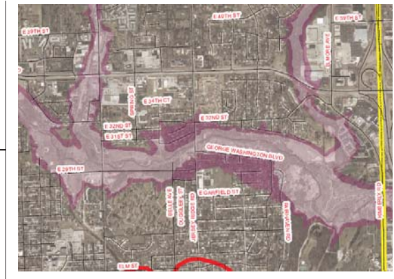
floodplain zoning prevents development from occurring in floodprone areas, as illustrated here for Duck Creek
